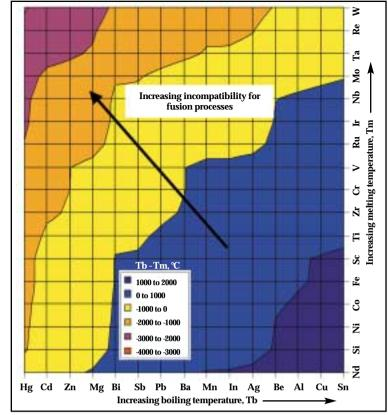
Fig. 4 — Some alloys are difficult or impossible to produce by fusion processes, because the melting temperature of one element may be greater than the boiling temperature of the other.
