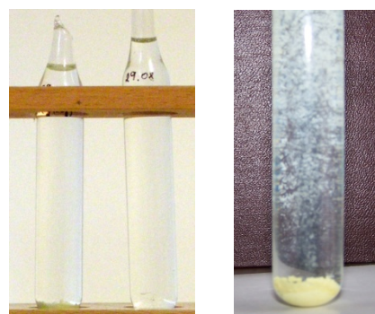
Figure 3. Left test tube: after another two and a half months the solution becomes colorless and clear and the sulfur completely precipitates at the bottom (see a better photo at the far right). No changes occur in the right test tube (the blank) containing only SO 2 (aq)
