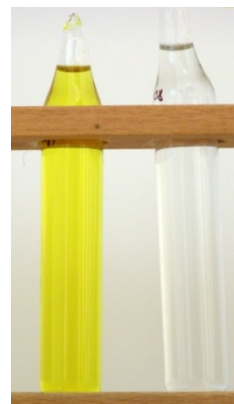
Figure 1. Left test tube: SO 2 dissolved in aqueous solution of potassium iodide; right test tube (a blank): SO 2 dissolved in distilled water
